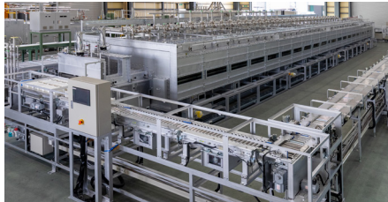
Roller hearth furnace
