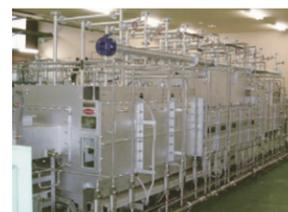
**Industrial furnaces for sintering lithium-ion batteries**
