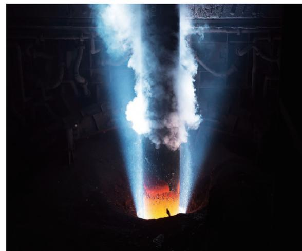
Graphite electrodes are used for melting iron scraps in EAF steelmaking. This method results in CO<sub>2</sub> emissions that are around one-fourth of those generated by the blast furnace method. The share of electric furnace steel is expected to increase to curtail environmental impacts, and mounting demand for graphite electrodes is anticipated.
